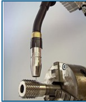
Figure 9: FRONIUS TransPuls Synergic 3200 CMT G/W – Application du CMT Pin www.alganmetal.com.tr
