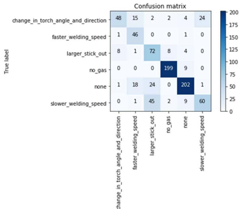
Figure 10: Prediction of the used welding conditions based on the AI model (Source : OQTON)
