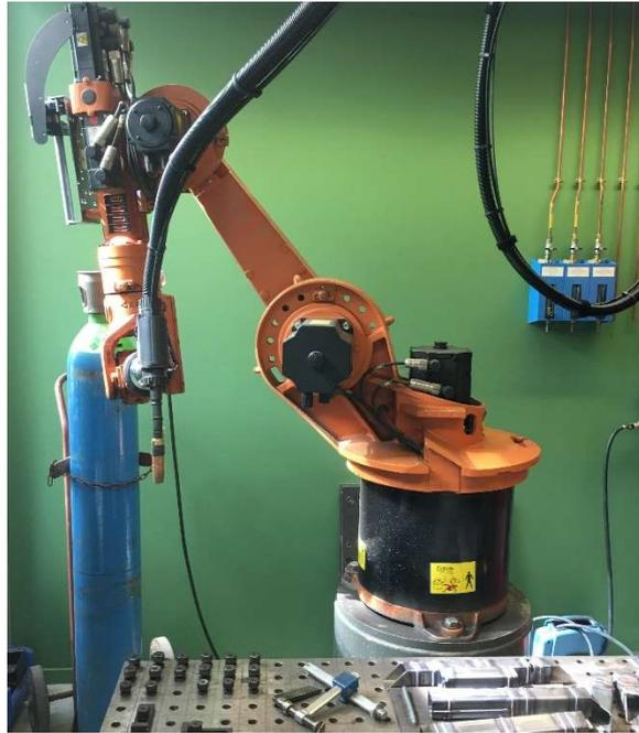
*Figure 4: Robot used to create the welds @ BWI*
