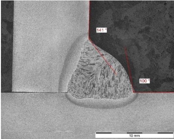
Figure 12: Cross section of weld FWa4-STA1
