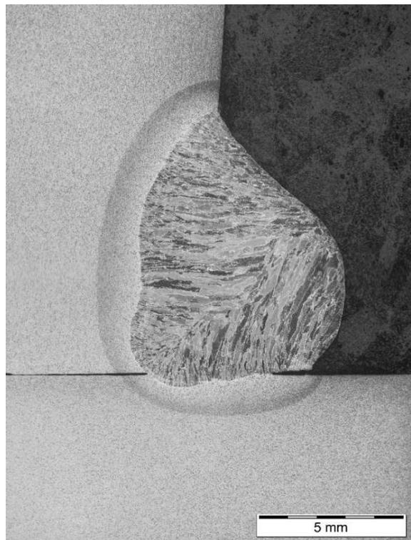
Figure 15: Cross section of weld FWa4-HA-5
