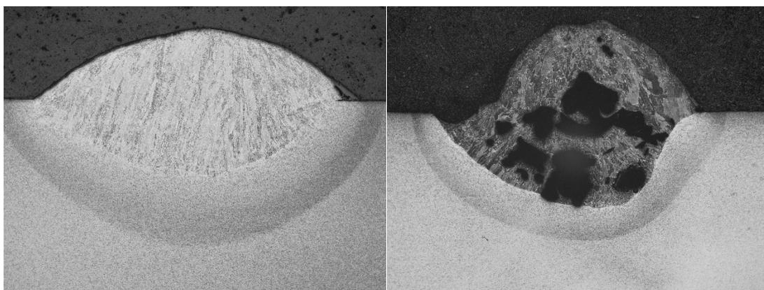
Figure 8 : Left: Cross-section of a weld (reference condition; spray arc welding)
