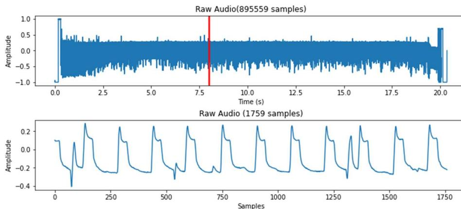
Figure 16 : Measured voltage signal of a high quality weld (FWa4-STA-1)
