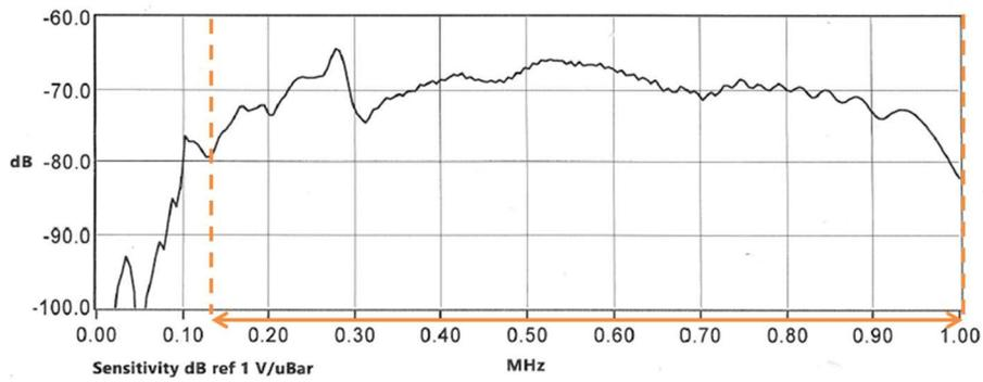
Figure 1: Wideband Differential (WD) sensor
