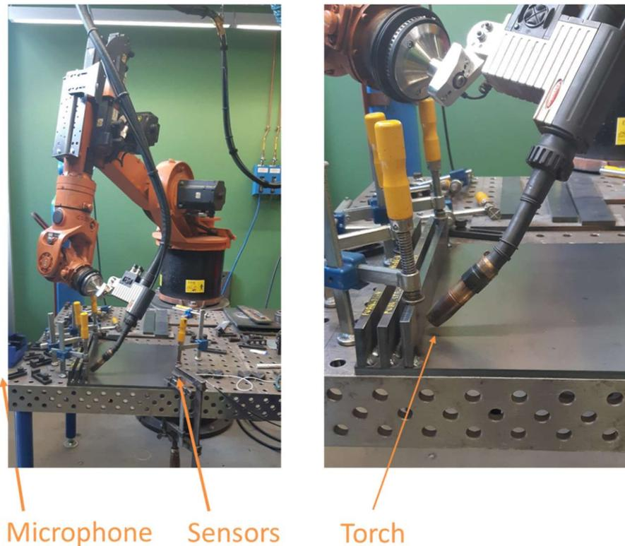
Figure 11: Test set-up used for fillet welds (Source : BWI)
