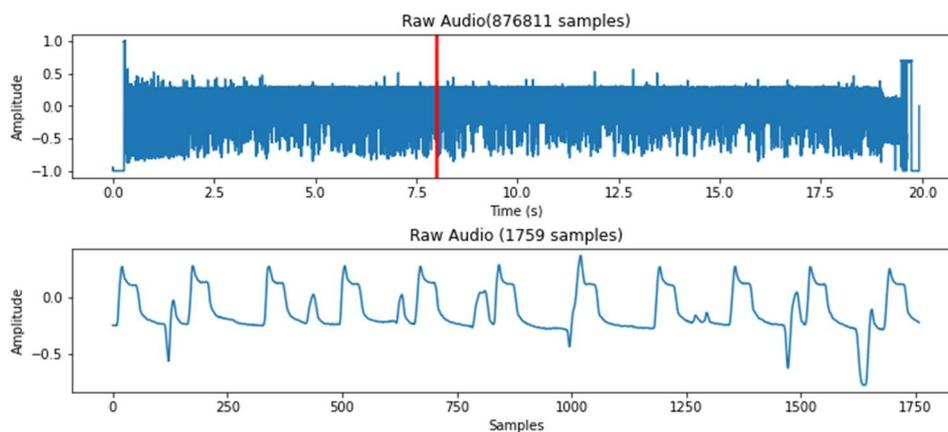
Figure 17: Measured voltage signal of a low quality weld (FWa4-STA-6) (Source : OQTON)
