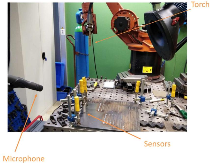
Figure 7: Test set-up used for the bead-on-plate welds (Source : BWI)
