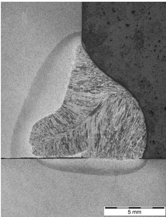
Figure 14: Cross section of weld FWa4-26-7
