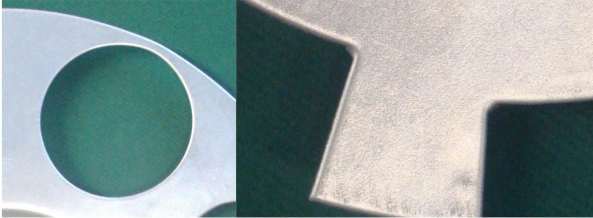
**Figure 15:** Left: Influence of neighbouring cutting elements. Right: Remaining radii in sharp edges
