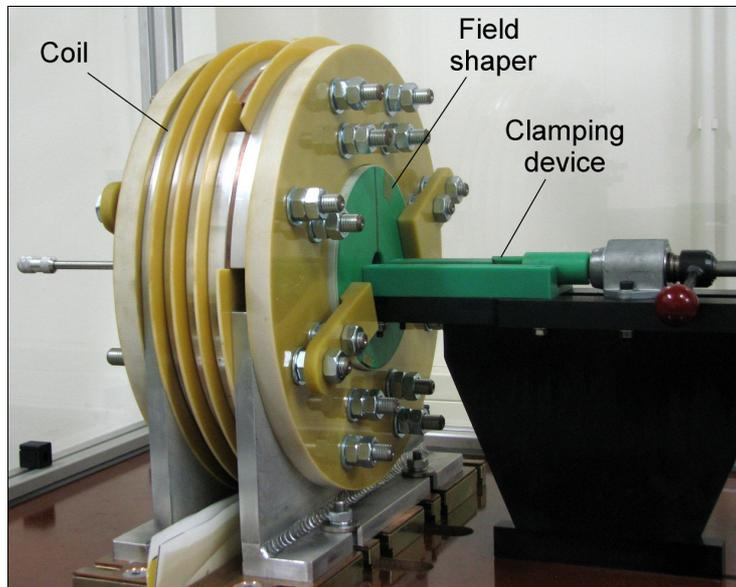
*Fig. 3: Multi-turn coil used in the experiments*
