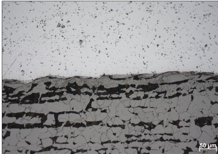
*Fig. 8: Flat weld interface of an aluminum-steel weld*
