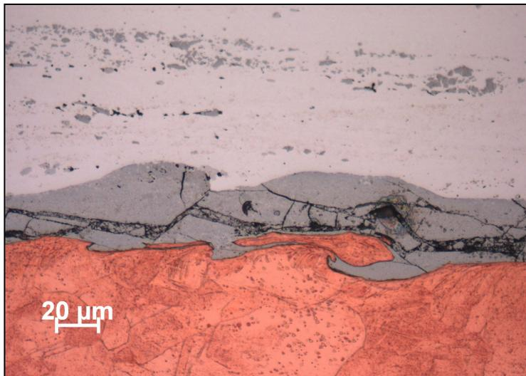
*Fig. 11: Cracks in the intermetallic layer of a copper-aluminum weld, executed at a too high energy level*
