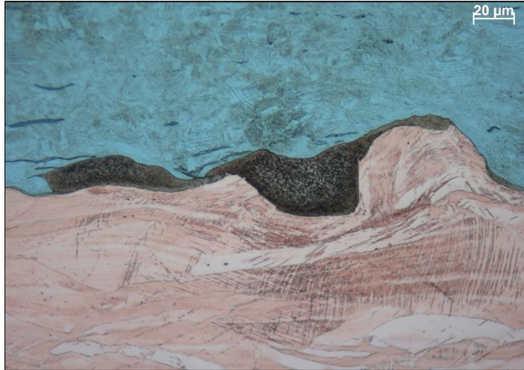
*Fig. 10: Large intermetallic layer observed in a copper-stainless steel weld, executed with a high energy level*
