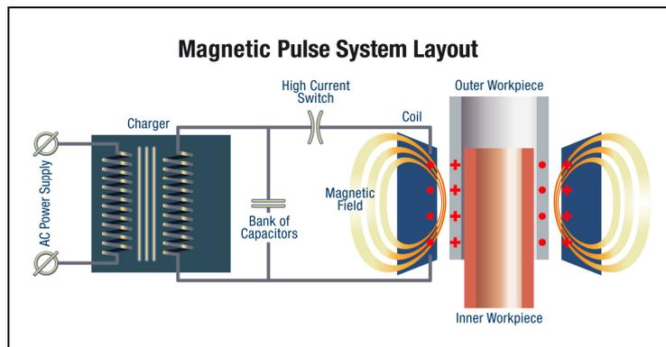
*Fig. 1: Principle of magnetic pulse welding [7]*
