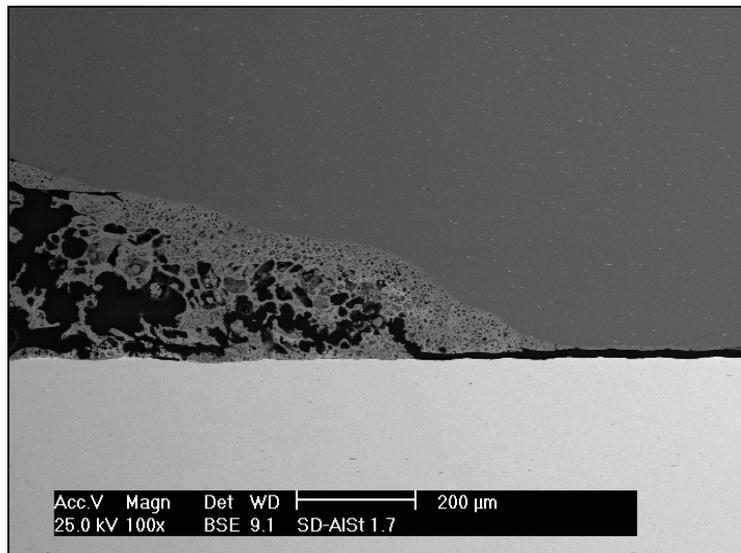
*Figure 16: Molten material in the run-out zone of an aluminum-steel weld*
