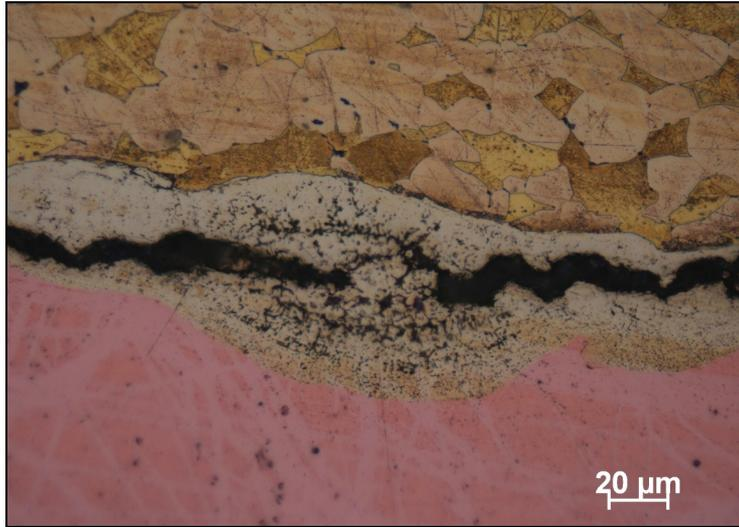
*Fig. 13: Molten zones with cracks along the weld interface of a copper-brass weld*
