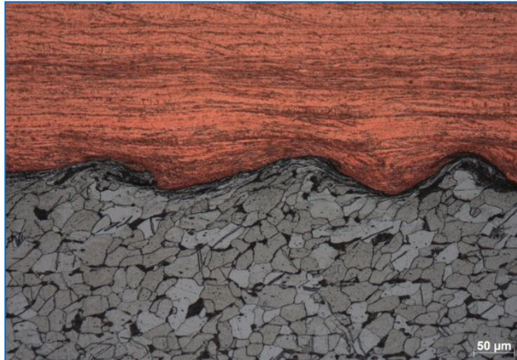
*Fig. 6: Wavy weld interface of a copper-steel weld (detail of figure 5)*
