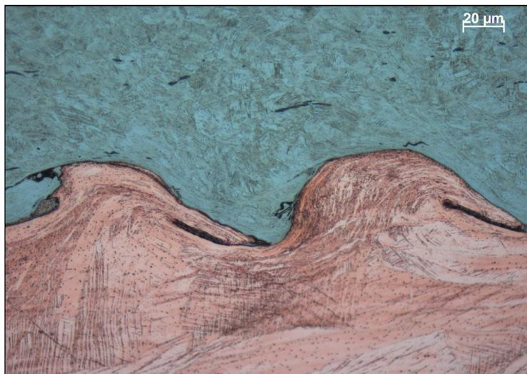
*Fig. 9: Thin intermetallic layer observed in a copper-stainless steel weld, executed with a low energy level*
