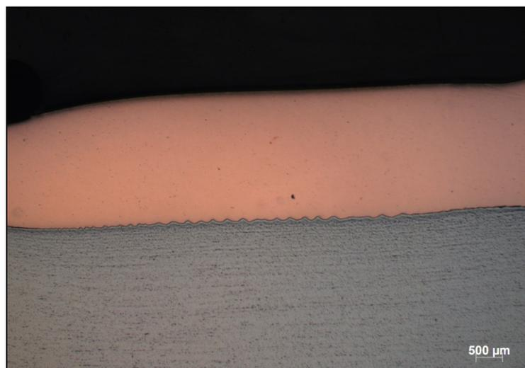
*Fig. 5: Metallographic section of a typical copper-steel weld*
