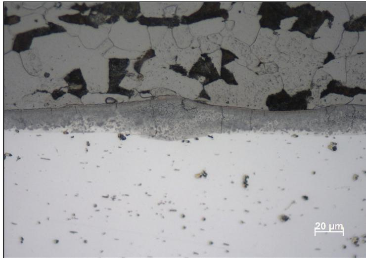
*Fig. 12: Vertical cracks in the intermetallic layer of an aluminum-steel weld*
