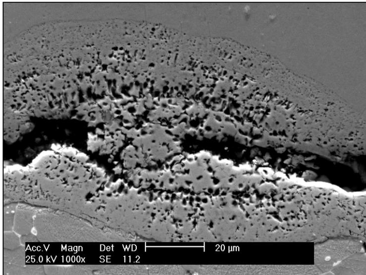
*Fig. 14: Scanning electron microscopic analysis of a molten zone in a copper-brass weld (detail of Figure 13)*
