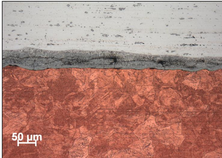
*Figure 15: Copper-aluminum weld interface with local melting*
