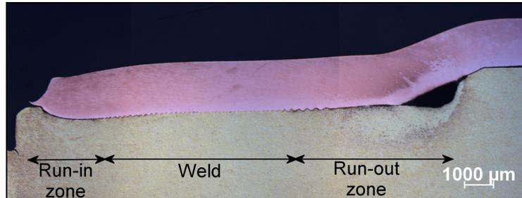
*Fig. 4: Metallographic section of a typical copper-brass weld*
