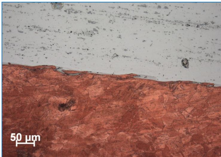
*Fig. 7: Weld interface of a copper-aluminum weld (with a small and flat intermetallic layer)*
