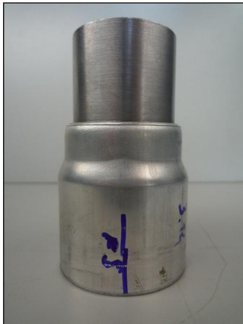
*Fig. 2: Aluminum-steel weld (tube diameter: 45 mm, wall thickness: 1,5 mm)*
