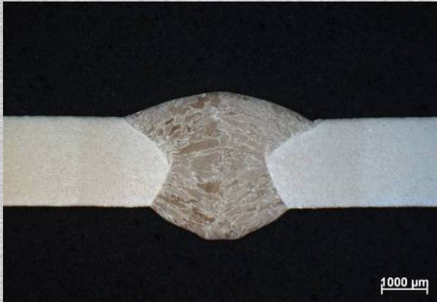
Figuur 1: DC01 (2 mm) - Conventioneel MAG
