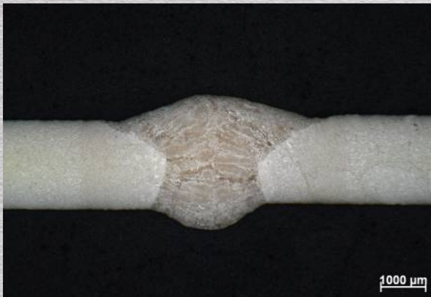
Figuur 4: DC01 (2 mm) - Cold Process (Cloos) Ar-18% CO 2
