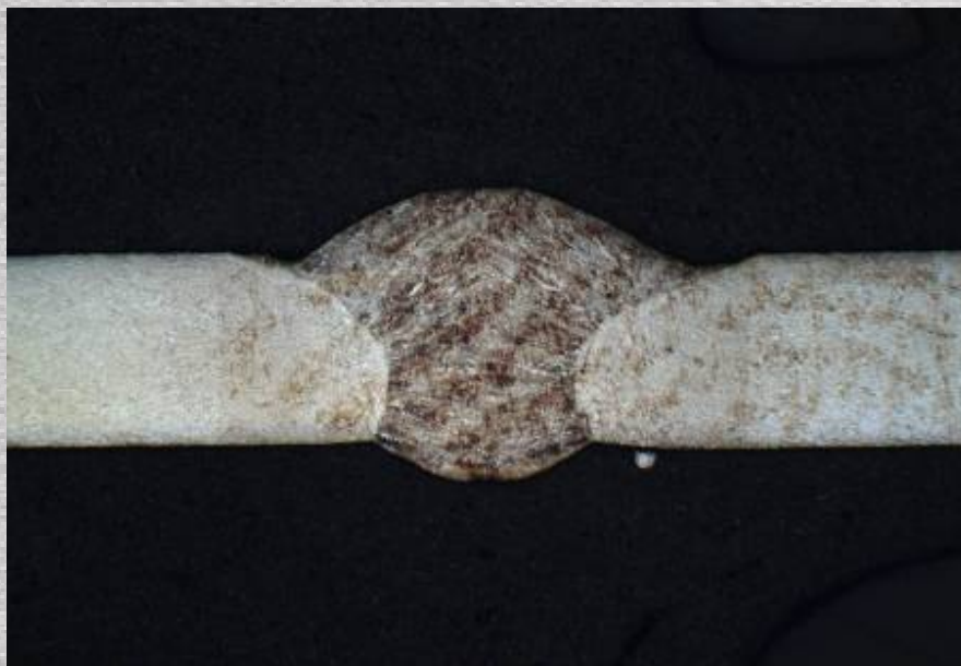
Figuur 2: DC01 (2 mm) - Cold Process (Cloos) Ar-15% CO 2
