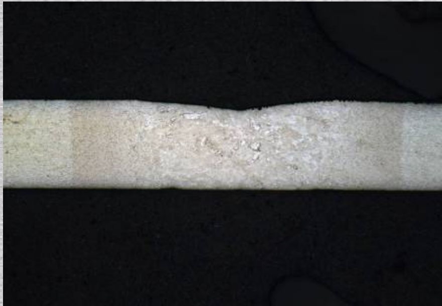
Figuur 7: DC01 (2 mm) - Conventioneel TIG
