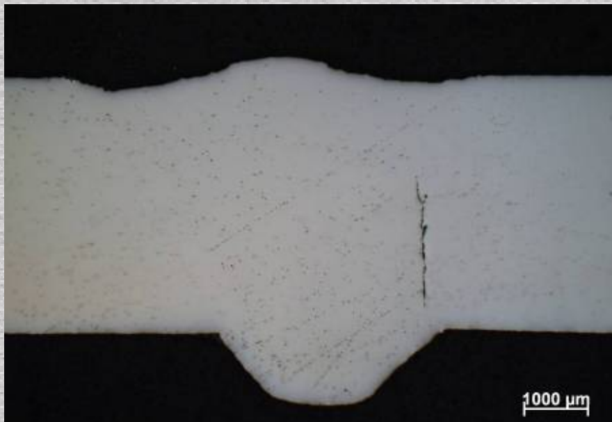
Figuur 8: S700MC (4 mm) - Conventioneel MAG (Afgekeurd wegens bindingsfout)
