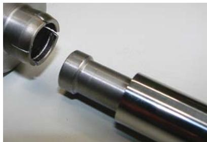
Figure 14: Tube with 4 cracks as a result of radial forces during relative sliding in the tensile test
