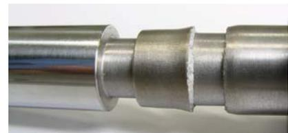
Figure 15: Shearing of tube metal during tensile test
