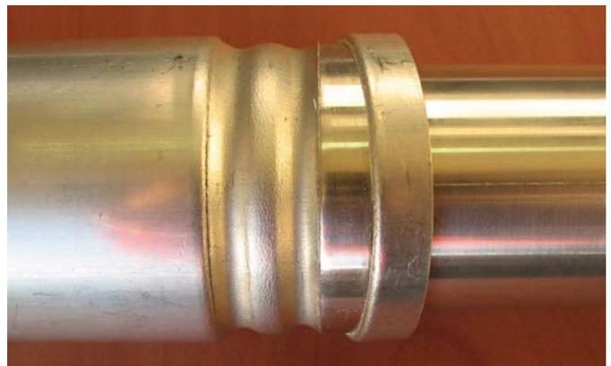
Figure 11: Mandrel with sharp edges cuts the tube
