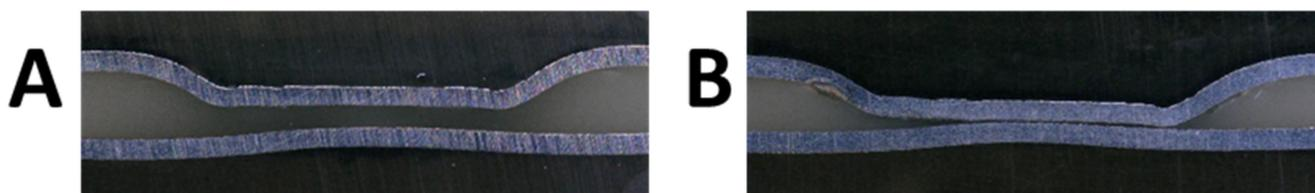
**Figure 10.** Selection of the induction preheating parameters: (A) too short time 20 s and (B) correct heating time 30 s.
