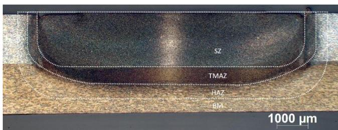
Figure 3: Cross-section of a friction stir spot weld with the associated zones [2].
