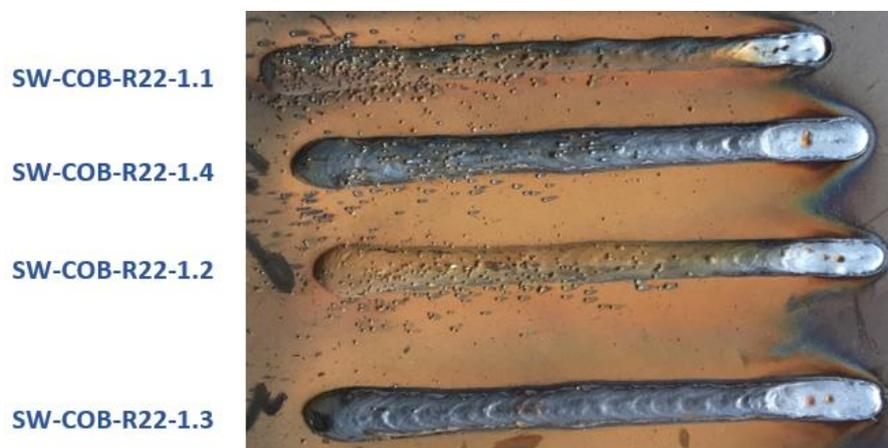
Figure 151: Visual inspection of the good quality arc welds in test series R22.
