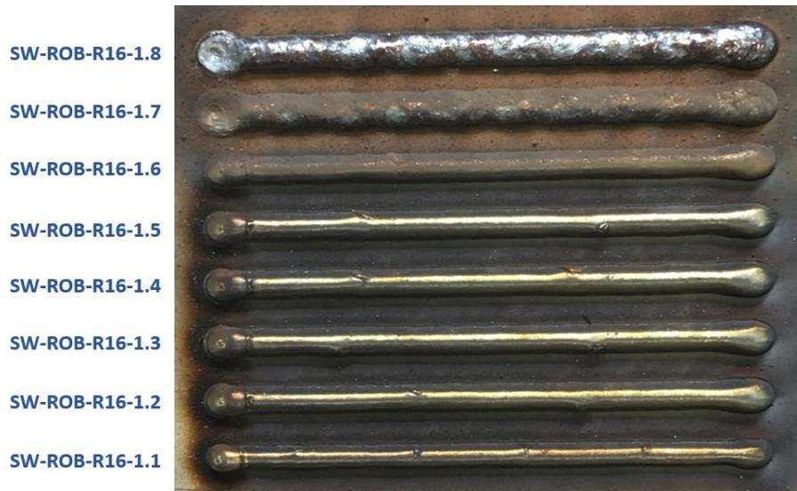
Figure 125: Visual inspection of the welds in test series R16.
