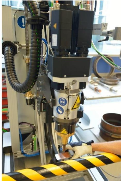
Figure 44: Used refill friction stir spot welding machine [4].
