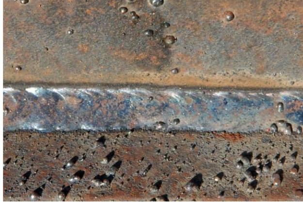
*Figure 28: Spatters as a welding defect [61].*
