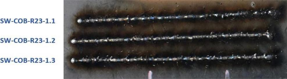
Figure 152: Visual inspection of the bad quality arc welds in test series R23.
