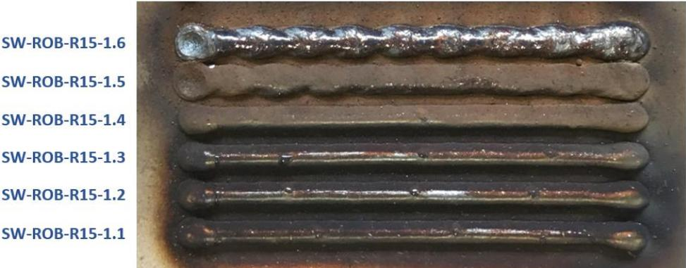
Figure 118: Visual inspection of the welds in test series R15.
