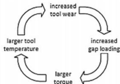
Figure 5: The wear problem with gap loading between the tool components [9].
