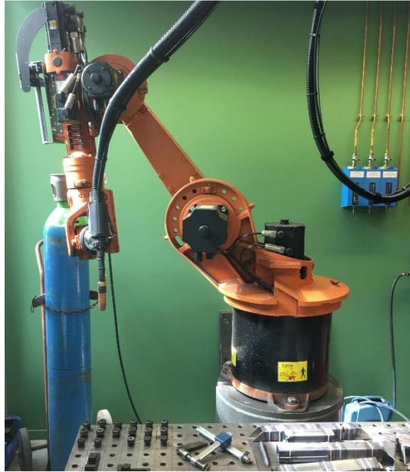
Figure 46: Used robot to create the arc welds discussed in this investigation.
