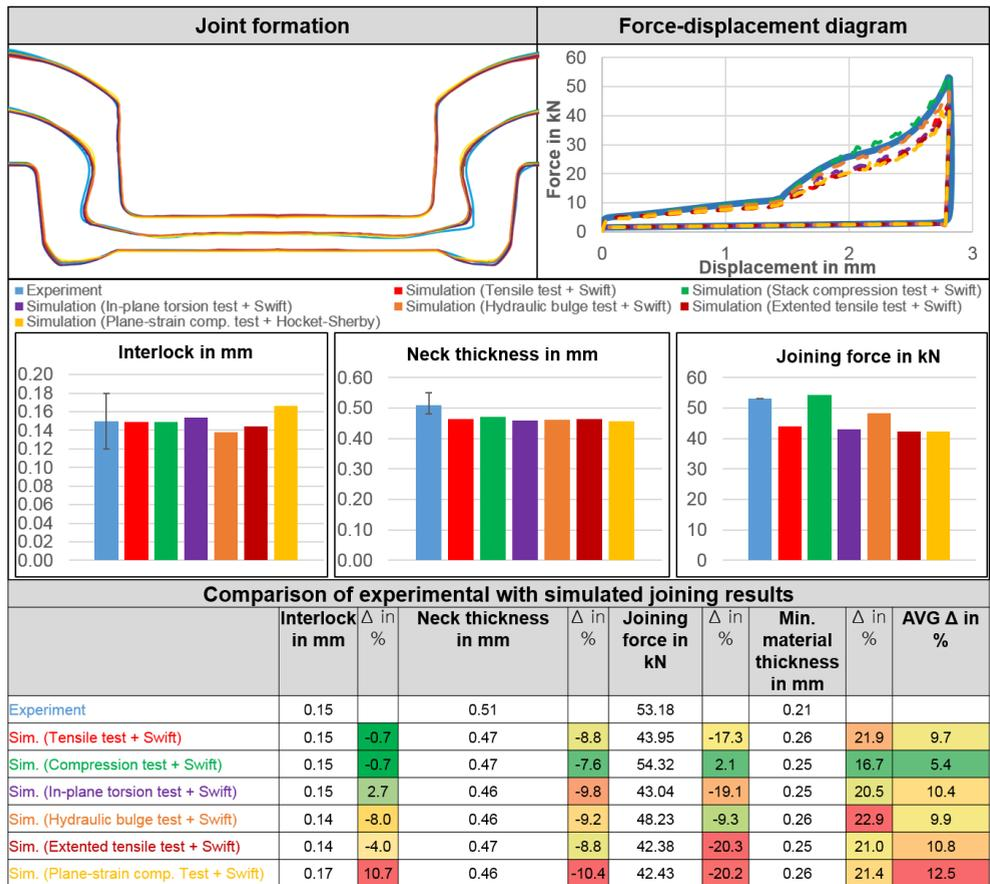
Figure 138: Comparison of simulation results with different flow curves for Clinching of DC04 ( $t = 1.0$  mm) in DC04 ( $t = 1.0$  mm)
