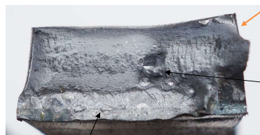
Lack of fusion
